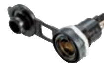
57607002 DIN Socket & Dust Cap 16A 12/24V DIN Plug with dust and splash proof cap Dust and splash proof socket Requires Ø 18mm opening
